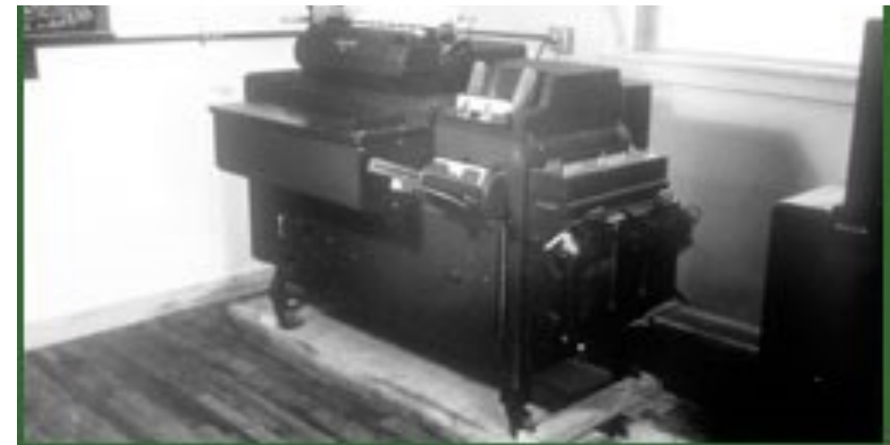
One of the first IBM card listing machines used at Los Alamos. During the war it was used primarily to perform the numerical calculations necessary to design the implosion device.
